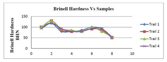
Figure 7.Brinell hardness test for Al 7075 hybrid metal matrix composites (Suryakumari et.al [11])
