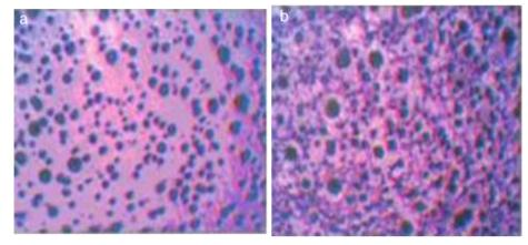
Figure 1.Optical micrograph of Al 2024/ (10% SiC + 10% fly ash) (a) before etching and (b) after etching (Boopathi et al. [2])
