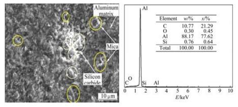
Figure 2.(a) SEM image of Al/10SiC-3mica composite(b)EDS spectrum of Al/10SiC-3mica composites (Rajmohanet al. [3])
