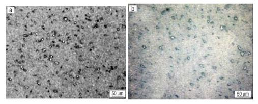
Figure4.Microstructure of surface hybrid composites (a) Al-SiC/Gr; (b) Al-SiC/Al<sub>2</sub>O<sub>3</sub> (Deravaju et al. [5]) Suryakumari et.al.[11] studiedAl7075 hybrid metal matrix composites (Al7075+ SiC + Al<sub>2</sub>O<sub>3</sub>) was produced via stir castingtechniques. Al7075 is a matrix material and SiC ,  $Al_2O_3$  are the reinforcing elements. The Al7075aluminium alloy with 2.5, 5 and 7.5 W% of SiC and 2.5, 5 and 7.5 W% of Al<sub>2</sub>O<sub>3</sub> was produced viastir casting.
